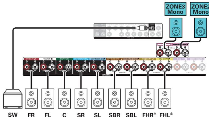
\* The height speakers, ceiling speakers and Dolby Atmos Enabled speakers can be connected to the HEIGHT1 speaker terminals. Set the speaker to be connected from "Speaker Layout" in the menu. (p. 230)
