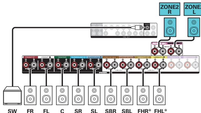
\* The height speakers, ceiling speakers and Dolby Atmos Enabled speakers can be connected to the HEIGHT1 speaker terminals. Set the speaker to be connected from "Speaker Layout" in the menu. (p. 230)
