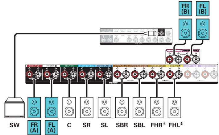
\* The height speakers, ceiling speakers and Dolby Atmos Enabled speakers can be connected to the HEIGHT1 speaker terminals. Set the speaker to be connected from "Speaker Layout" in the menu. (p. 230)
