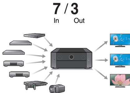
This unit is equipped with 7 HDMI inputs enabling connection to various HDMI compatible devices such as Blu-ray Disc players, game consoles and HD video camcorders. There are dual HDMI outputs for the main room, and a third HDMI output for another room.
