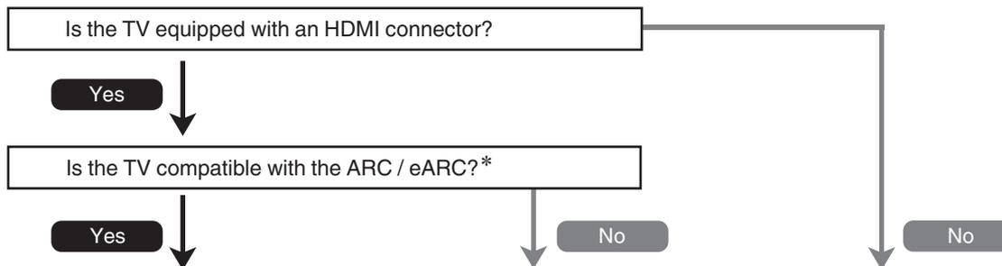
**“Connection 1 : TV equipped with an HDMI connector and compatible with the ARC / eARC”** (🔧 p. 76)
