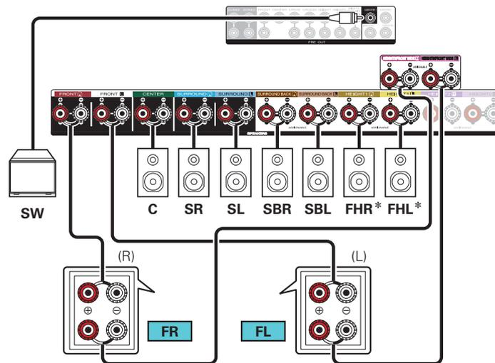
\* The height speakers, ceiling speakers and Dolby Atmos Enabled speakers can be connected to the HEIGHT1 speaker terminals. Set the speaker to be connected from "Speaker Layout" in the menu. (p. 230)
